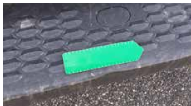
Stigbrett bak: Liten deformering
